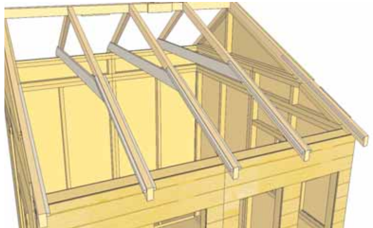
46. Position 3/4" x 3/4" x 44" long Lexan Support Cleats on each Long Rafter flush to end and recessed 3/16" down from top of rafter. Nail to rafter using 6 - finishing nails. Note, Start nails in Supports on ground first. Complete remaining 7 Lexan Support Cleats.
