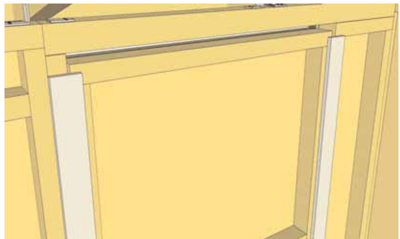
69. Attach Interior Door Stops to door framing from inside of shed. Start by securing both Vertical Door Stops . Use Horizontal Door Stop to help determine distance between vertical stops. See Step 70 for detail. Use 4 - 2" screws to secure each Stop. Stops should overlap door by approx. 1/2".
