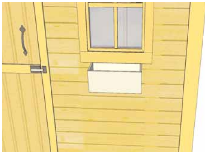
73. Attach Window Box below bottom of window trim with 2 - 2" screws. Screw from inside of box into the center wall stud. Attach second screw 2" below top screw.
