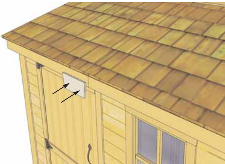
72. Attach Facia/ Detail Plates to cover seam where Front Facia pieces come together. Secure 4 - 1 1/2" finishing nails .
