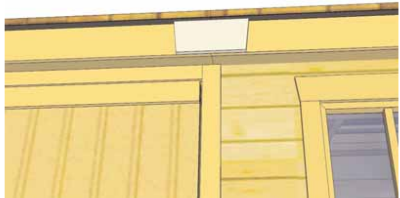
72. Attach Facia/ Detail Plates to cover seam where Front Facia pieces come together. Secure 4 - 1 1/2" finishing nails .
