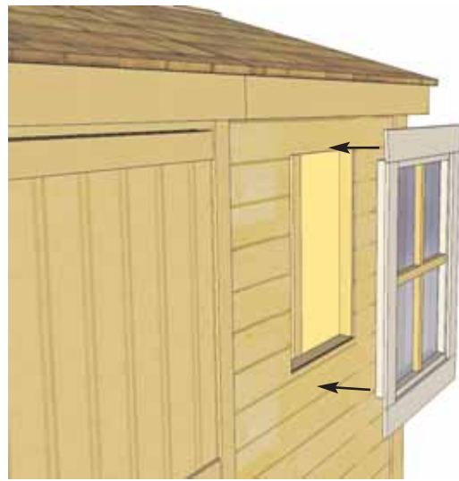
67. Locate Window Insert and place in window wall cavity.
