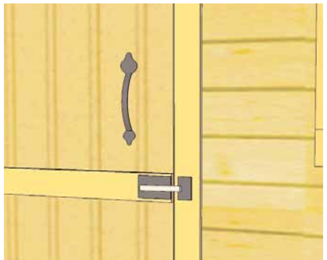
71. Attach Door Handle and Exterior Barrel Bolt . Handle is positioned on top part of door. Barrel Bolt should be positioned on middle door trim and narrow trim. Use hardware provided in each kit.
