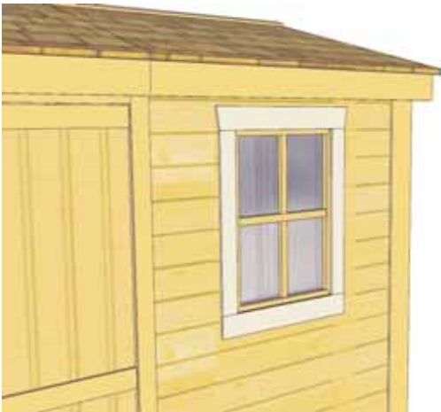
68. Place Window Insert into opening. Push so window trim sits flush against wall siding. On the inside, shim Window Insert evenly in cavity. SpaceSaver kits include one additional shingle for shimming of the window. When properly positioned, secure Window Insert to wall framing cavity with 4 - 2" screws.
